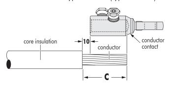
B. Remove the core insulation from the conductor for a distance **« C »** mm
