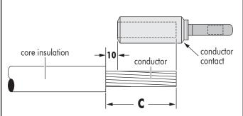
A. Remove the core insulation from the conductor for a distance **« C »** mm
