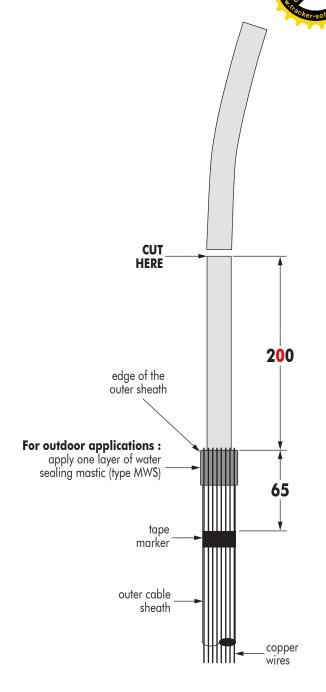
**3 For indoor applications**, bend the screen wires back over the outer sheath and proceed to step no. 4.
